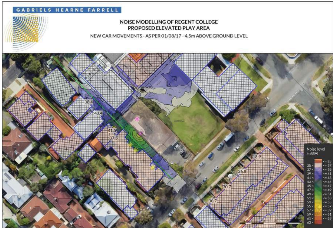
Image 05 - Noise Emissions from New Vehicle Movements - Receivers at 4.5m above ground level
