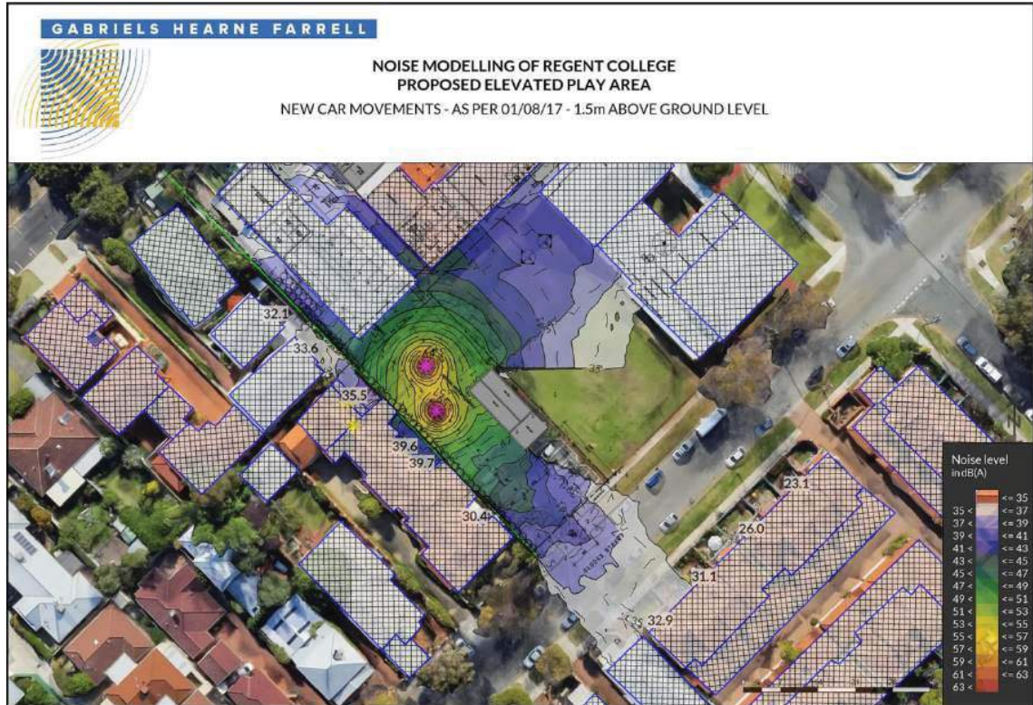
Image 04 - Noise Emissions from New Vehicle Movements - Receivers at 1.5m above ground level
