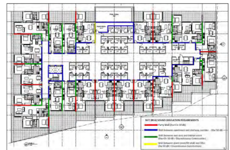
Figure D3: Wall mark-up for Level 2
