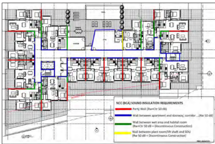
Figure D4: Wall mark-up for Level 3
