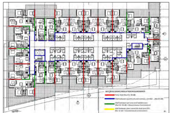
Figure D2: Wall mark-up for Level 1
