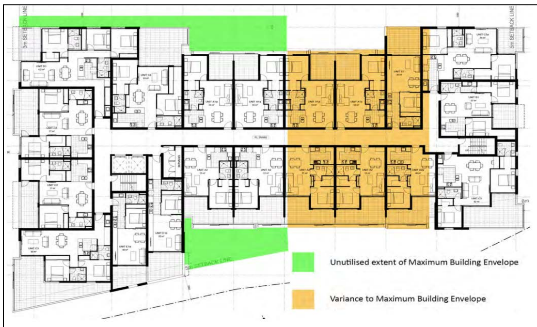
Figure 11 – Variation to maximum building envelope
